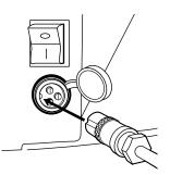
**1** Plug the charger port into the port on the scooter. The charger works with the power switch in either the on or off position. The charging input, on/off switch and overload breaker are located under the deck at the front left-hand side.
